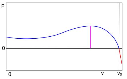
Above graph really challenges Lorentz force based explanation of the rotating magnetic field's drag, but we can assign this discrepancy to the increase of inductive resistance of the medium that follows increase of the frequency. Another less straight explanation is that the image of the magnet is slightly affected by the Doppler's effect that distorts the image canceling the drag force.
