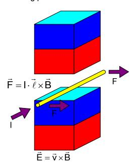
Above picture shows a lateral force acting to the wire with the current.
